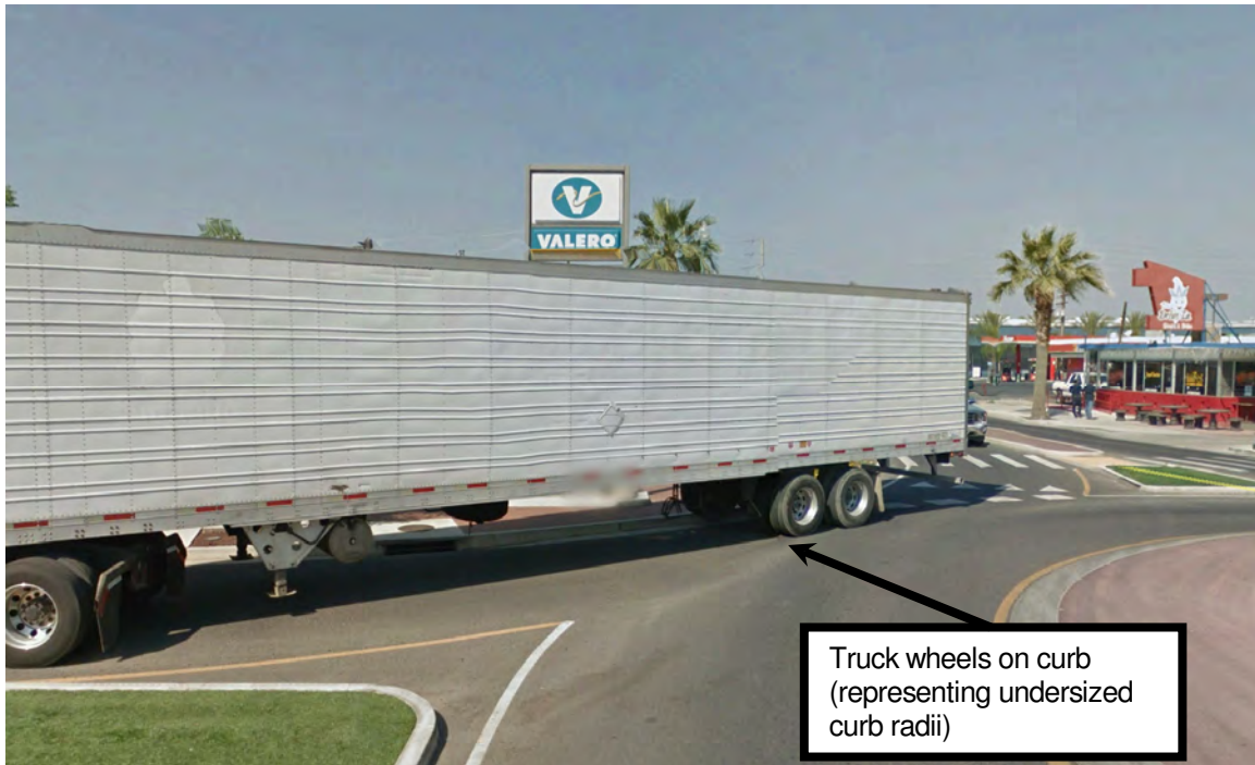
Figure C - Truck driving on undersized curb radii
